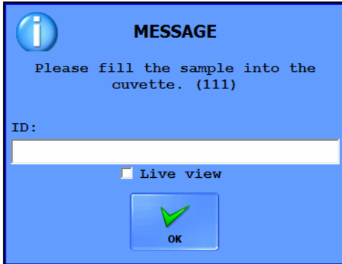
Fig. 35: The Live View checkbox appears with the Please fill sample into cuvette message, if you enabled the function in the Measure tab
