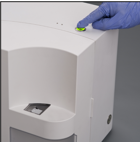
Fig. 29: The Start button on the top of the analyzer is the only interface element you need: press it once and the system feeds a cuvette into pipetting position.
