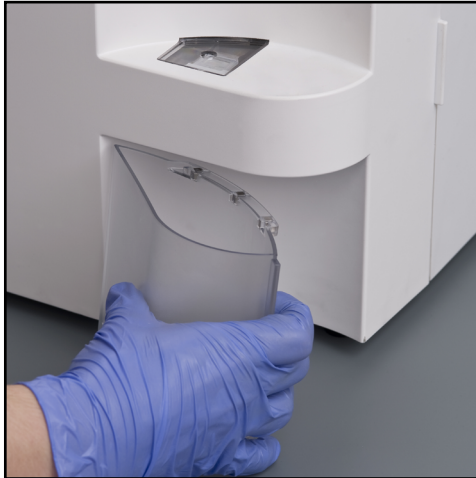
Fig. 33: Do not leave any used cuvettes in the waste drawer at the end of the day. Use the overhanging flap of the waste drawer to grip it and take it off the analyzer.
