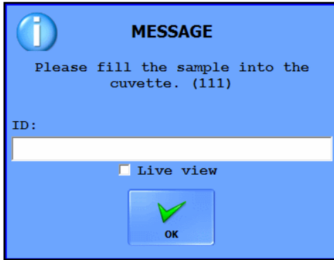
Fig. 30: When the cuvette is in the pipetting position, a message prompt appears. Scan the barcode or type in ID. Click OK and push the start button again to start cuvette processing.
