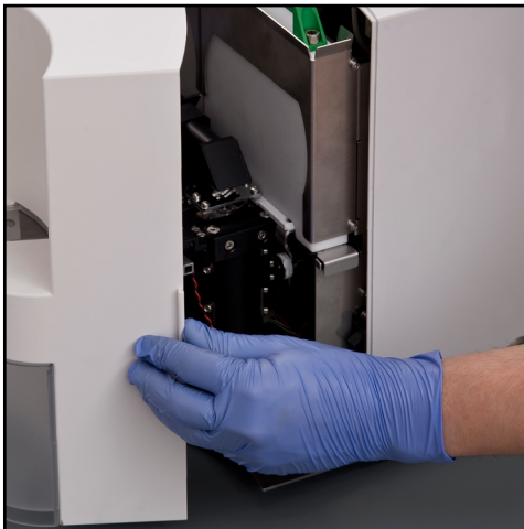
Fig. 27: Open the analyzer door to access the cuvette holder slot
