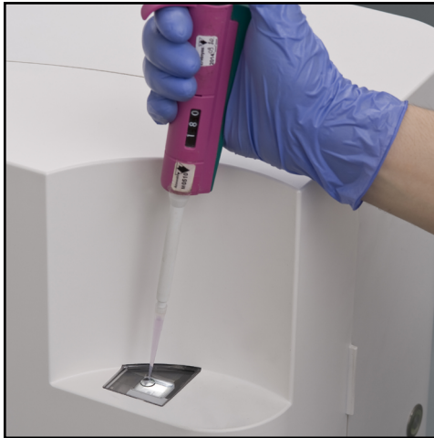
Fig. 31: The backlighting under the see-through plastic cuvette helps you guide the tip of the pipette for fast and efficient work
